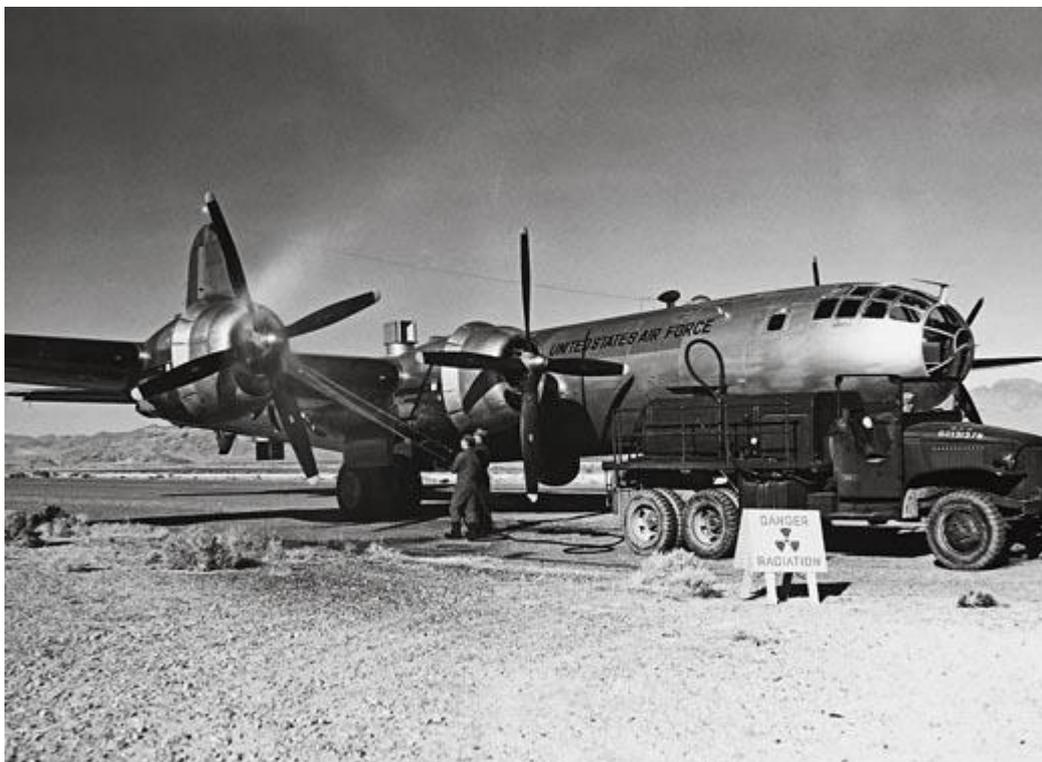
*Air Force personnel decontaminate a B-29 sampler aircraft with Gunk degreaser. Photo, probably taken in early 1950s, provided by National Nuclear Security Administration / Nevada Site Office and reproduced in Mark Wolverton, "Into the Mushroom Cloud," Air and Space Magazine July 2009.*
